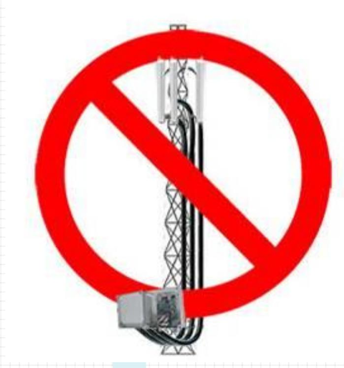
Tree or four high loss cables (RGC213, LMR400), 6 or 8 conectores and antennas very close together.
