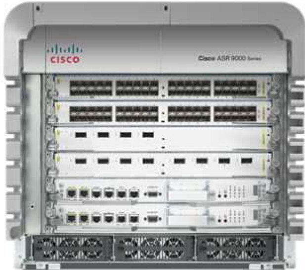
Cisco ASR 9006/10 Router
